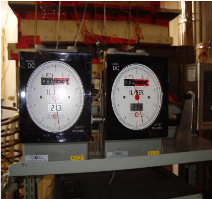
Picture 11: Dry gas meter
