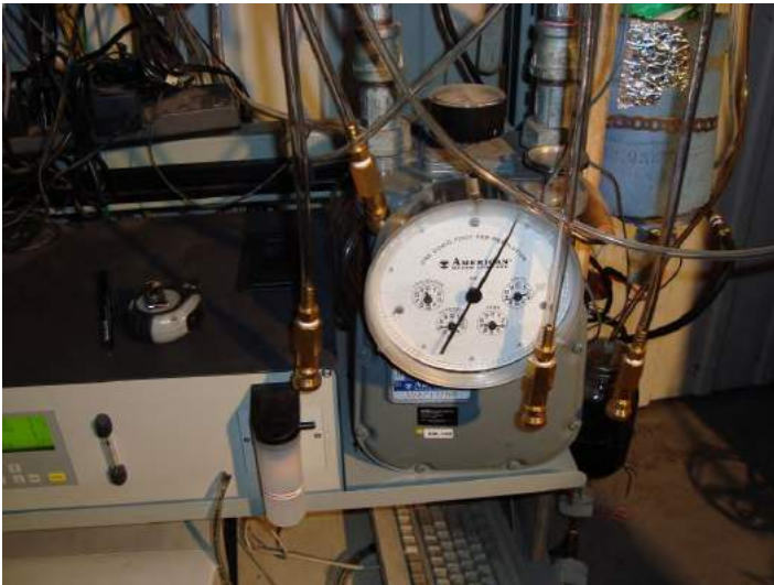
Picture 8 : Reference dry gas meter
