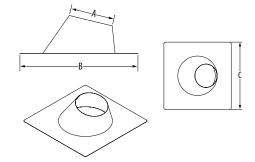
Use to weather-proof the penetration of the galvanized outer jacket through the roof. Made of galvalume.
