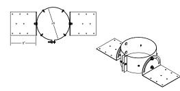
Used to support galvanized outer jacket and PolyPro vent within at the roof level. Adjustable to different roof pitches. Ideal for cathedral ceilings.
