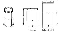
Adjustable Adapter with flange for galvanized outer jacket. Flange attaches to appliance cabinet with supplied screws. To calculate installed length, subtract 1 1/2" for each joint.
