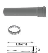
Use to vent condensing appliances. 2" (60mm) of overlap at the joint. Listed to ULC S636. Locking Clamps are required at all joint connections. Includes 1 Locking Clamp per each length. Sold in full box quantities only.
