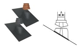
Use to weather proof penetration of vent through the roof. For concentric pipe. Made of polypropylene. Adjusts from 5/12 to 12/12. Black or terra-cotta. UV resistant.
