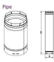
Galvanized outer jacket can be used as a conduit for single-wall PolyPro pipe. In exterior applications, provides protection from impact and UV light. Also provides some insulation value for use in colder climates. Can be field-painted if desired. Simple twistlock assembly. To calculate installed length, subtract 1 1/2" for each joint. Includes internal metal support ring. PolyPro pipe sold separately.
