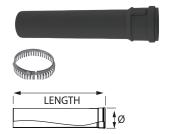
Use to vent condensing appliances. 2" (60mm) of overlap at the joint. Listed to ULC S636. Made of UV resistant polypropylene. Includes 1 Locking Clamp.
