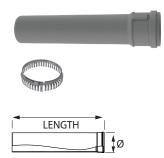
Use to vent condensing appliances. 2" (60mm) of overlap at the joint. Listed to ULC S636. Locking Clamps are required at all joint connections. Includes 1 Locking Clamp per each length .
