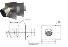
Use for through-the-wall horizontal terminations. Includes 23 degree termination elbow with integrated bird screen, inner and outer wall plates, and clamp for connecting to PolyPro pipe. No locking Clamp is required. All components are stainless steel.
