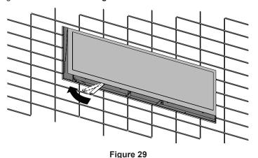
**NOTICE:** The glass door is secured to the top of the firebox with tabs that allow the glass door to pivot outward at the bottom. The bottom of the door frame engages into the four bullet type retainers.
