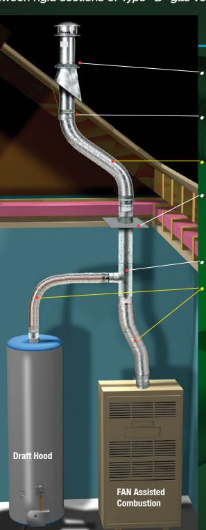
Rain Cap, RV Pipe, Storm Collar, Adjustable Flashing
