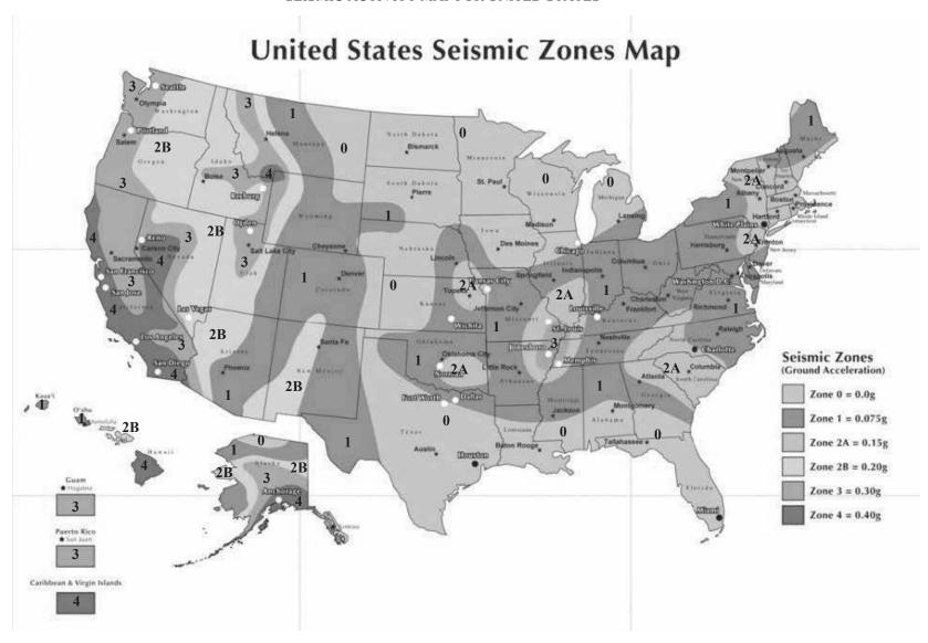
Mason-Lite Fireplaces have been tested and passed the seismic requirements for Modular Masonry Fireplaces throughout the entire United States. We understand that not every installation needs the extra security that is involved in a high seismic zones. Rebar is ONLY REQUIRED in Mason-Lite units in seismic zones 3 & 4 shown in the map below. We will supply rebar to all fireplaces shipped to in the United States unless otherwise requested.
