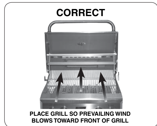
Fig. 10-2 Airflow direction - CORRECT
