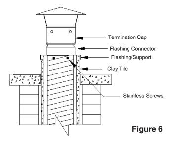
**.7** Install the Termination Cap by lining up the prepunched holes in the cap and the Flashing Adaptor. Secure in place with Stainless Steel screws (not supplied).
