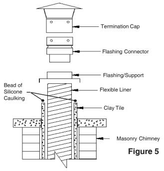
.2 Pull enough of the Flexible Liner out of the chimney to enable you to apply a bead of RTV Silicone caulking into the Flexible Liner 1" from the top edge of the liner.
