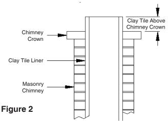
Remove Clay Tile Above Chimney Crown If Damage is Evident
