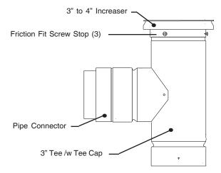
Figure 7b - Assembled components
