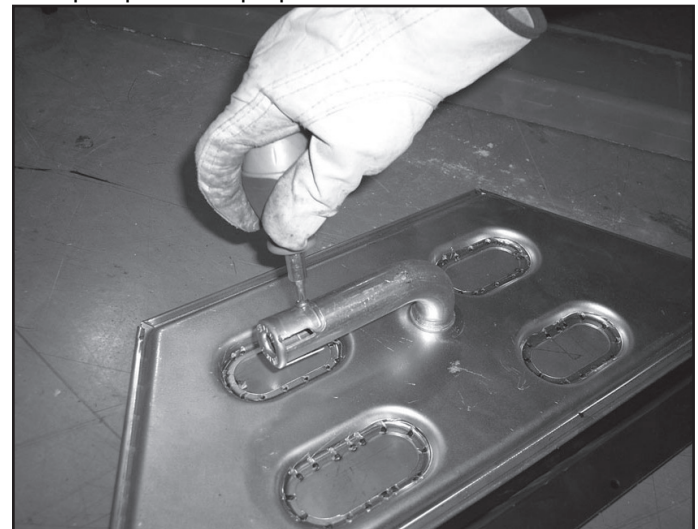
Figure 14.31 Adjust Air Shutter
