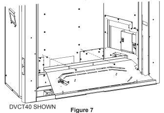
4. Remove Blower Access Plates by taking out (6) screws each. See Figure 8.
