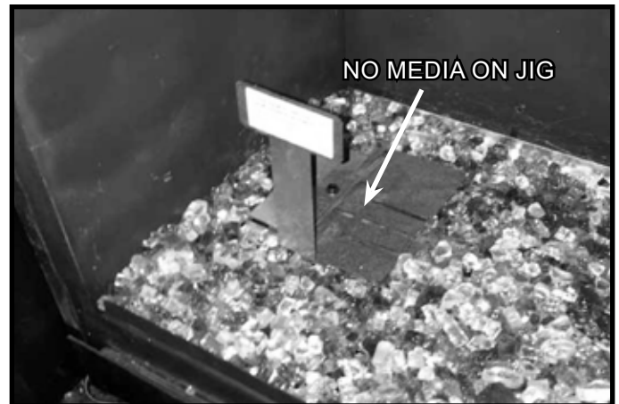
Figure 2. Media Placement Jig in Place
