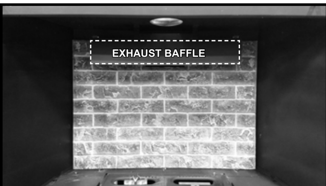
Figure 6. Install Back Refractory Panel
