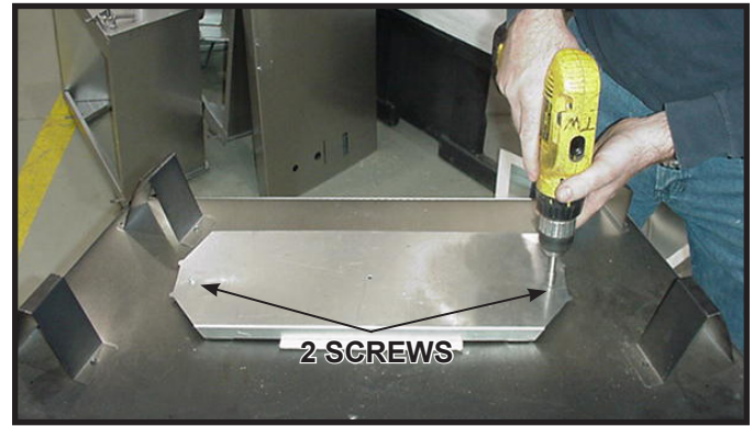
Figure 6.5 For top vent, remove the two screws holding the top heat shield in place. For rear vent, see next page.
