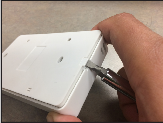
Figure 2. Wall Switch Disassembly
