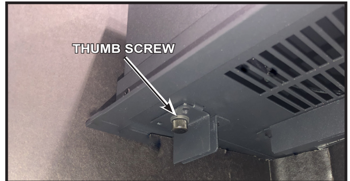
Figure 4.16 Glass Removal and Installation
