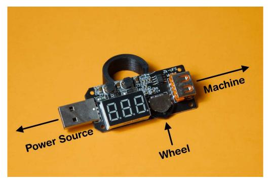
Plug the controller into a power source and the machine. The display will display the current output voltage
