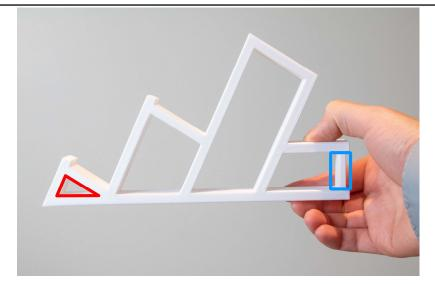
These are the places where the connectors are attached, red for the front connector, and blue for the back connector.
