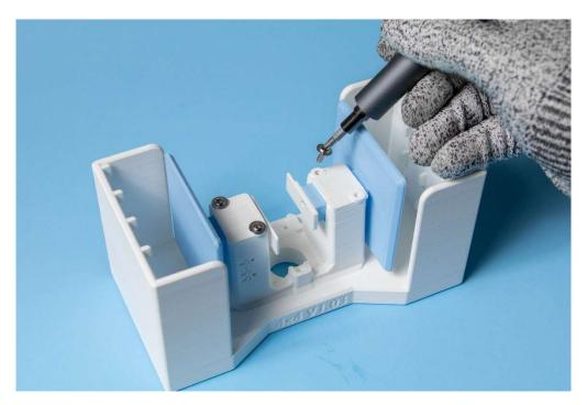
Step 3: reattach the cover piece. After tightening the screws, make sure the pusher assembly is able to move back and forth smoothly. If you experience increased friction than before, loosen the screws a bit and try again.
