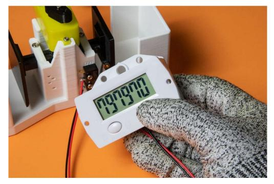
Step 9: Long press the RESET button to reset the counter, the counter resets itself after the count reaches 1,000,000.
