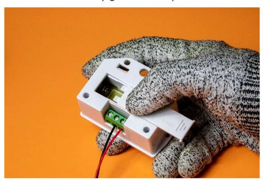
Step 6: Remove the battery compartment cover.
