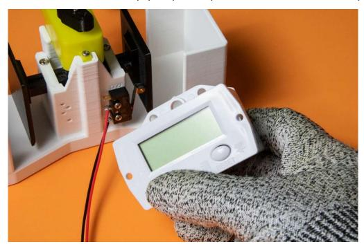
Step 8: Long press the POWER button (left) to turn on/off the counter. The current count will be saved when the counter is shut off.
