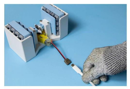
Step 3: Simply plug in the machine to start. To achieve consistency, it is recommended to break in switches by amount of time (min, hrs, etc).
