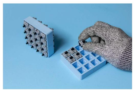
Step 1: Install switches into <u>both sides</u> of the switch plates (32 max on each).
