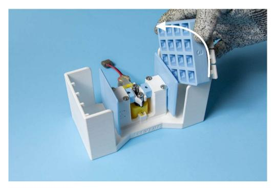
Step 4: Turn on the machine, the pusher will break in only one side of the switch. In order to break in the other three sides, rotate the switch plate 90 degrees after one side is finished. Please take notes on which side(s) has been broken in. 4 sides are labeled with numbers. For consistent results, break in each side for the same amounts of time.
