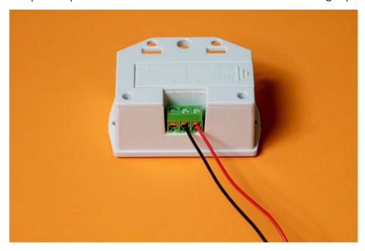
Step 2: Insert the 2 wires into the <u>right and middle</u> slots, the order of the wires does not matter. Make sure the screws are loose if you are unable to insert the wires.
