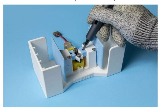
Step 1: Unscrew the screw holding in the buffer piece. The screw hole is designed to be at an angle, please angle the screwdriver as shown when removing the screw.
