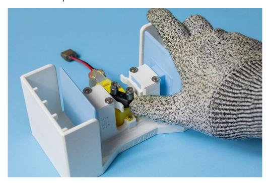
The wheel can be rotated when inserting the switch plates. Rotate the wheel SLOWLY and ONLY WHEN NEEDED to avoid breaking the gears. If the wheel can't be rotated in one direction, try the other. If both directions don't work, turn it on/off briefly and try again.
