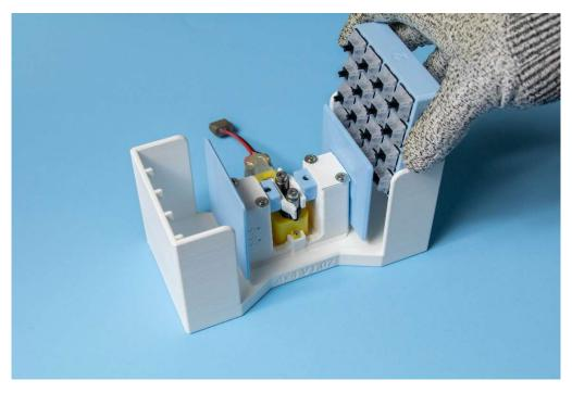
Step 2: Insert switch plates in any orientation. Switch plate orientation does not affect break-in process in Mode A.
