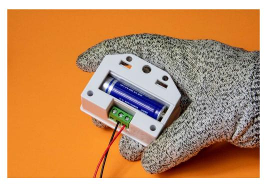
Step 7: Insert a AA battery (1.5v) and put the cover back in place.
