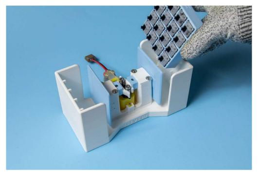
The switch plate is inserted through the top of the machine. The product will function with 1 or 2 plates, but operation with 2 plates is <u>highly recommended</u> (also make sure the 2 plates have the same amount of switches).
