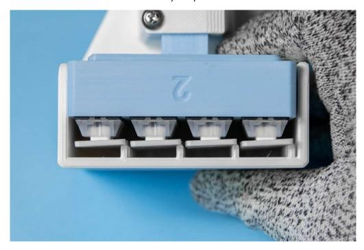
At this point, the user's machine should look like the image above. Once turned on, the nibs will apply a force to the side of the keycaps, resulting in more friction towards the side.
