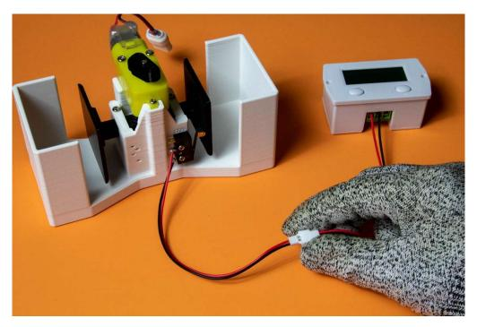
Step 5: Connect the two wires with the white connector, the pins only go in one way.
