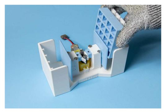
Step 3: Insert switch plates with the keycaps facing <u>away</u> from the pusher, the off-center nibs should line up with the edge of the keycaps
