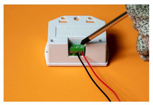
Step 3: Tighten the two screws and make sure the wires are secure.
