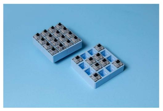
Make sure to space out the switches evenly if you are not planning on filling the entire plate. If you are filling the entire plates with switches, ~70g max bottom out switches is recommended.
