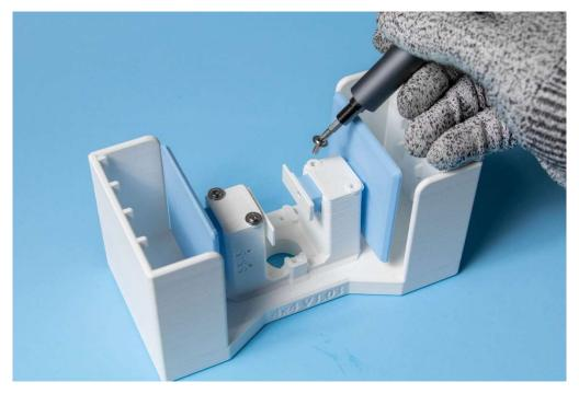
Step 3: reattach the cover piece. After tightening the screws, make sure the pusher assembly is able to move back and forth smoothly. If you experience increased friction than before, loosen the screws and try again.
