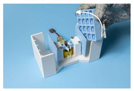
Step 4: Turn on the machine, the pusher will break in only one side of the switch. In order to break in the other three sides, rotate the switch plate 90 degrees after one side is finished. Please take notes on which side(s) has been broken in. 4 sides are labeled with numbers. For consistent results, break in each side for the same amounts of time.
