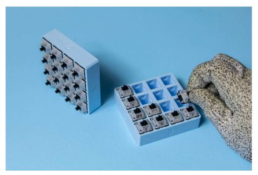
Step 1: Insert switches into <u>only one side</u> of the switch plate (16 max on each).
