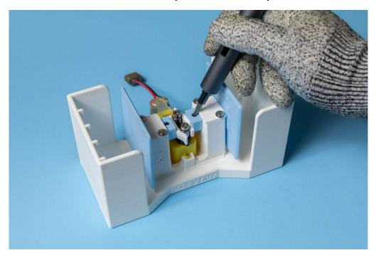
Step 1: Unscrew the screw holding in the buffer piece. The screw hole is designed to be at an angle, please angle the screwdriver as shown when removing the screw.
