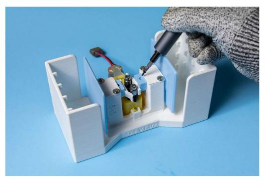
Step 3: Reattach screw. Again, the screwdriver needs to be at an angle as shown. If you find this difficult, feel free to remove the wheel before replacing the buffer pieces.
