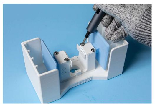
Step 1: Remove the pusher cover piece by unscrewing the top screws
