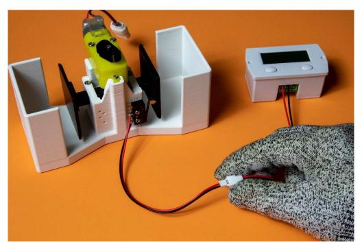
Step 5: Connect the two wires with the white connector, the pins only go in one way.
