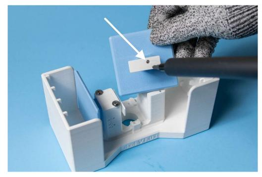
Step 2: Remove the screw holding the buffer piece in place. Replace the worn out buffer piece with a new one, and reattach the screw. Make sure to lubricate the surface where the bearings touch the buffer piece.
