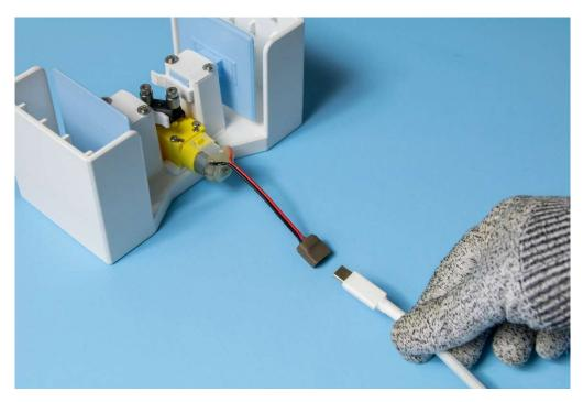
A standard 5V USB wall plug is recommended, along with any USB type-c cable. Simply plug or unplug the cable into the connector to turn the machine on or off. The user can also choose to use power banks or computer USB ports to provide power.
