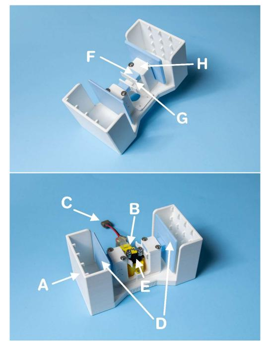
A: Main body B: Gear box C: Female USB type-c port D: Pusher plate E: Wheel F: Pusher G: Bearing-pusher buffer piece
