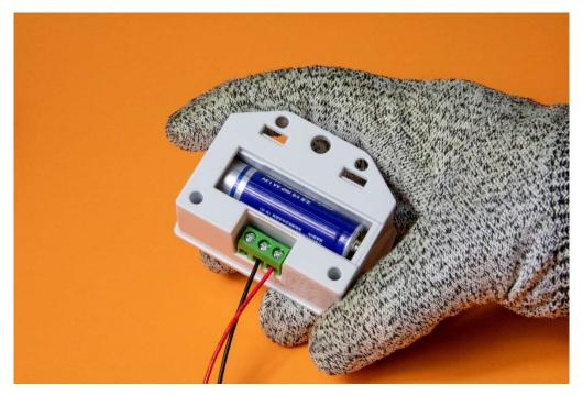
Step 7: Insert a AA battery (1.5v) and put the cover back in place.
