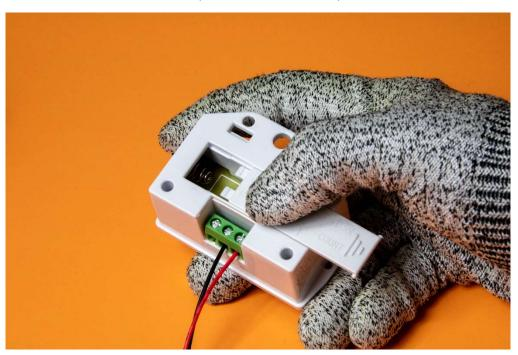
Step 6: Remove the battery compartment cover.
