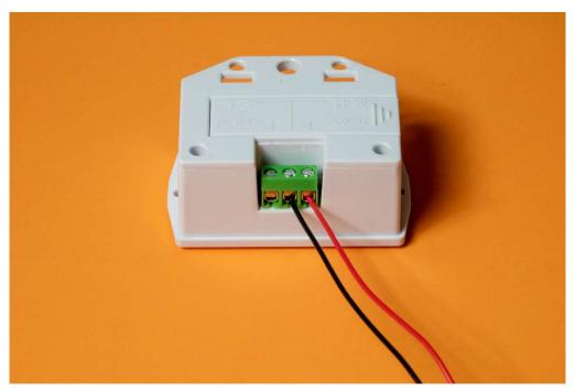
Step 2: Insert the 2 wires into the <u>right and middle</u> slots, the order of the wires does not matter. Make sure the screws are loose if you are unable to insert the wires.
