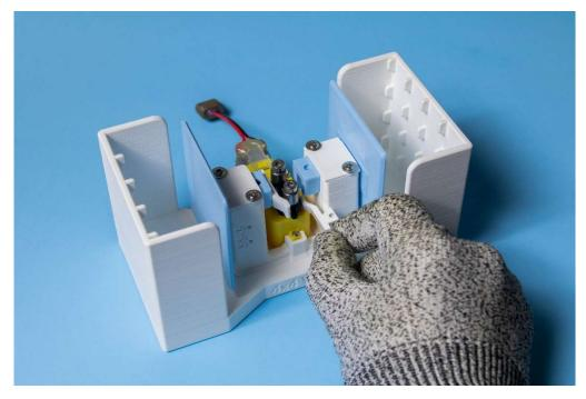
Step 2: Slide the worn out buffer piece downwards to remove it. Then replace it with a new one, make sure to lubricate the surface where the bearings touch the buffer piece with any grease.
