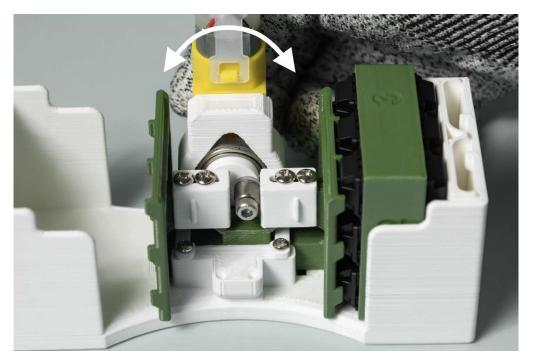
Step 3: Rotate the wheel as shown so that the switches are in the bottomed-out position. If you cannot move the wheel to the bottom out position, that means you need to lower the travel distance. (Note: the card is not shown in this picture, but it still needs to be inserted at this point)
