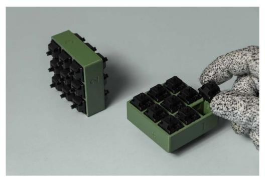
Step 1: Install switches into <u>both sides</u> of the switch plates (18 max on each plate).
