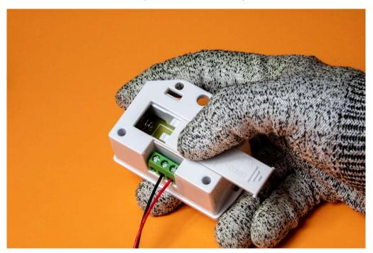
Step 6: Remove the battery compartment cover.
