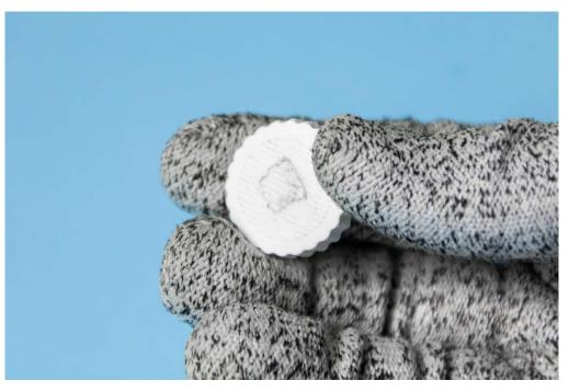
When to replace the buffer? Wear on the buffer will decrease the travel distance of the pushers, when this happens, sometimes one can compensate by adjusting the travel distance following section 6. Use your judgement, the pictured piece was used for ~400 hours and is still usable (picture from 4x4).
