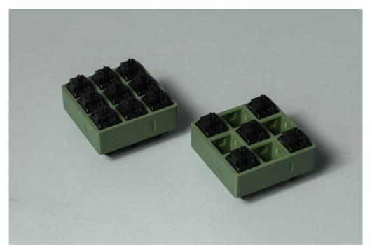
Make sure to space out the switches evenly if you are not planning on filling the entire plate. If you are filling the entire plates with switches, =<80g bottom out weight switches is recommended.
