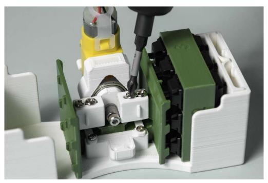
Step 1: Unscrew the 2 screws holding down the buffer. These do not need to be unscrewed completely, only loosened to allow the buffer to move. Note that the machine is adjusted for 4mm switches out of the box, unless you are using long pole switches, you do not need to adjust the travel distance. <u>This section needs to be done in mode A,</u> with no keycaps and the centered-mode spacers inserted.
