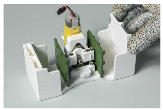
Step 2: Insert centered-mode spacers on both sides as shown.
