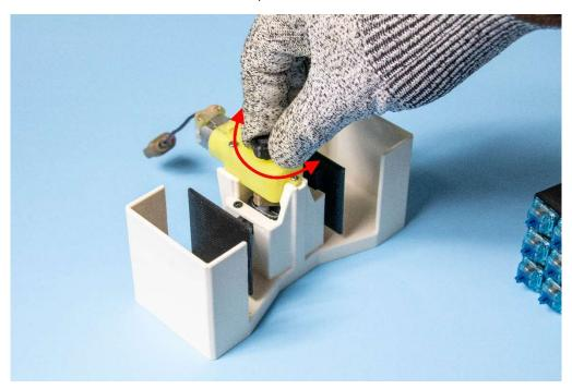
The top handle can be rotated to move the pusher plates when inserting the switch plate. When inserting the right plate, rotate the handle to move the pusher to the left most position. The opposite applies for the left plate. Rotate the handle SLOWLY and ONLY WHEN NEEDED to avoid wearing down the gears. The gear box is not designed to be rotated manually.
