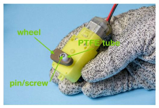
Step 3: Flip the gear box assembly, exposing a wheel, screw (this is the pin) and a PTFE tube surrounding it.
