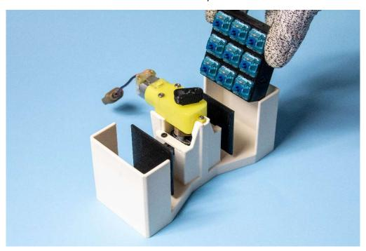
Step 2: Insert switch plate(s) in any orientation. Switch plate orientation does not affect break-in process in Mode A.
