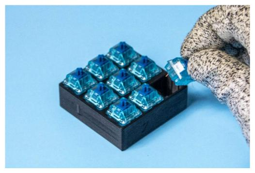
Step 1: Insert switches into only one side of the switch plate(s) (9 max on each).
