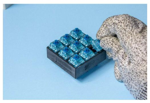
Step 1: Install switches into **both sides of the** switch plate(s) (18 max on each).
