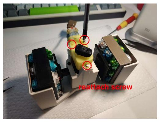
Step 11: Reattach the 3 screws that was removed in step 1.
