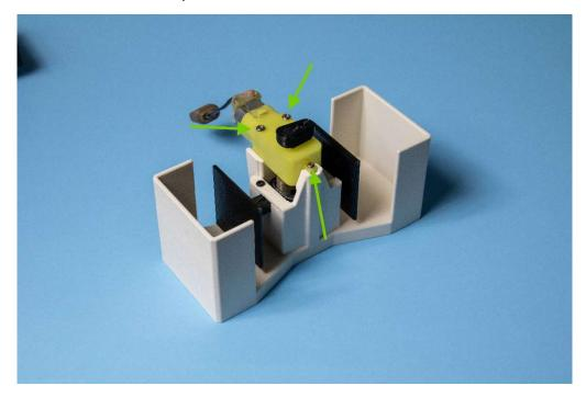
Step 1: Unscrew the 3 screws indicated in the picture above. Do so slowly to avoid stripping the plastic.
