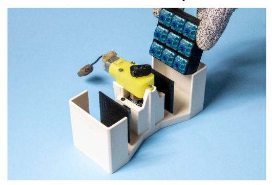
The switch plate is inserted through the top of the machine. The product will function with 1 or 2 plates.
