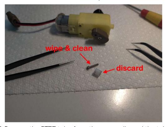
Step 5: Remove the PTFE tube from the screw, discard the tube and wipe the screw to get rid of any remaining lubricants and/or plastic bits.
