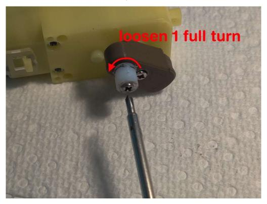
Step 9: Loosen the screw by 360 degrees (1 full turn counterclockwise) so that the tube is allowed to spin freely.
