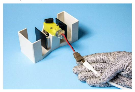
A standard 5V USB wall plug is recommended, along with any USB type-c cable. Simply plug or unplug the cable into the connector to turn the machine on or off. The user can also choose to use power banks or computer USB ports to provide power.
