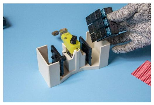
Step 5: Turn on the machine, the pusher will break in only one side of the switch. In order to break in the other three sides, rotate the switch plate 90 degrees after one side is finished. Please take notes on which side(s) has been broken in. 4 sides are labeled with numbers. For consistent results, break in each side for the same amounts of time.
