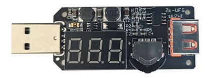
Plug the controller into a power source and the machine. The display will display the current output voltage
