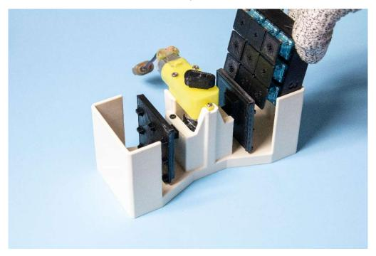
Step 4: Insert switch plate(s) with the keycaps facing the pusher, the 9 protrusions on the off-center actuation module should line up with the bottom edge of the keycaps. Insert spacers on the underside of the switch plate if needed.
