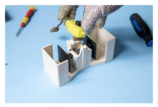
Step 2: Lift up the entire gear box assembly, including the top handle and the power cable. The pusher assembly should still remain in place.
