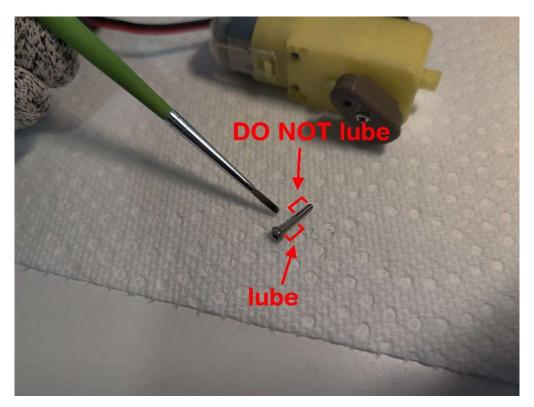
Step 6: Apply a thin coat of grease to the screw, DO NOT apply it to the part where the screw screws into the wheel. This can be any form of grease (krytox, tribosis, dielectric, etc), thicker is better.
