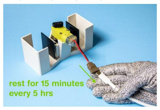
To prevent overheating and potential fire hazards, please DO NOT leave the product operating unattended. It is also highly recommended to pause the machine for ~15min after operating for 5hrs. This is to allow for the motor to cool down and to increase longevity of the product.
