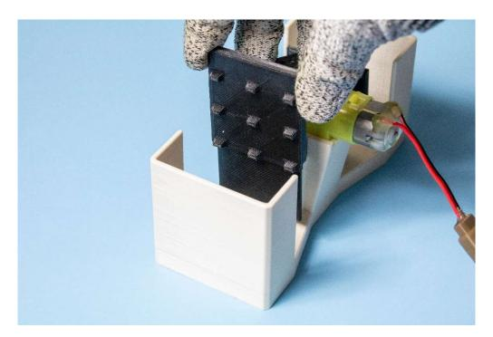
Step 3: Insert off-center actuation module onto the pusher plate by orienting the clip opening downwards, and sliding it on from the top.
