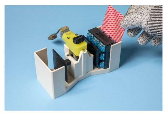
Step 3: Insert card stock spacers between the outer switches and main body if needed. A small space needs to be left in order to prevent jamming.
