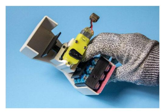
Card stock spacers are placed on the inner side of the main body. The purpose of spacers is to fill in empty spaces to ensure that the switches bottom out properly. Only insert spacers when machine is turned off. Rotate the top handle to the left/right most position while switches are installed to ensure there are no empty gaps.
