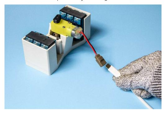
Step 4: Simply plug in the machine to start. To achieve consistency, it is recommended to break in switches by amount of time (min, hrs, etc).
