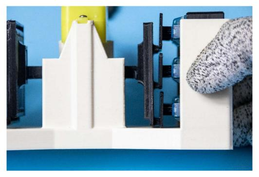
At this point, the user's machine should look like the image above. Once turned on, the pusher will apply a force to the side of the keycaps, resulting in more friction towards the bottom side.
