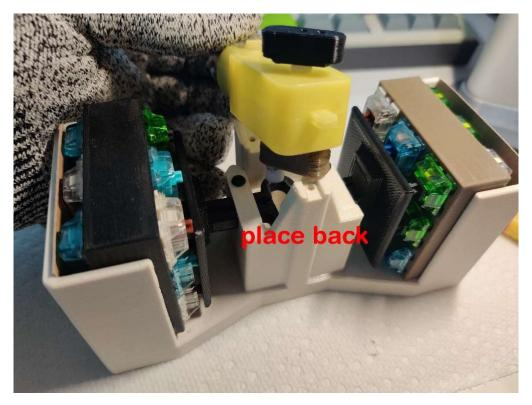
Step 10: Place the gear box assembly back onto the main body, make sure to line up the pin with the slot on the pusher.
