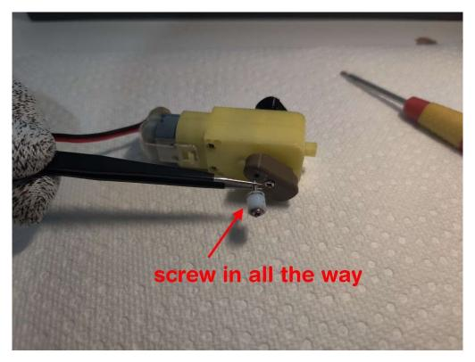
Step 8: Screw in the PTFE tube and pin assembly back onto the wheel so that the wheel does not spin freely when touched (the screw does NOT tighten all the way), do so slowly to avoid stripping the plastic.
