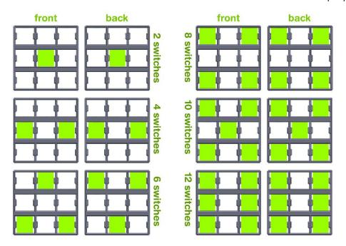
When operating in mode A with less than 18 switches on a plate, space out the switches evenly to ensure an even amount of pressure is applied to each switch. A minimum of 2 switches is needed on a plate.
