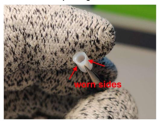
As the machine operates, the PTFE tube on the pin for the scotch yoke will wear out and side(s) will become thinner as the material grinds away. The tube will need to be replaced when the thinnest point is <0.5mm thick.
