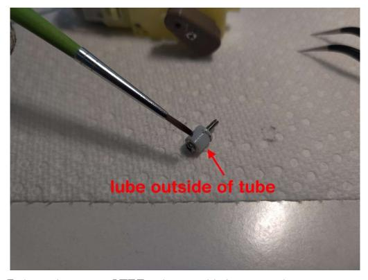
Step 7: Attach a new PTFE tube and lubricate the exterior of the tube with grease.
