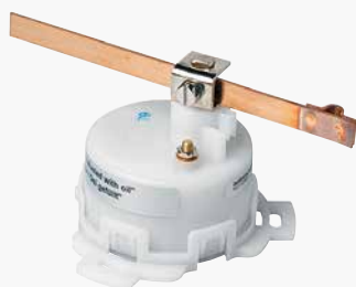
Rudder Angle Sensor
