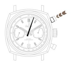
To reset the chronograph, press the reset pusher. The chronograph hand will jump back to the 12 position ('instant reset' function).
