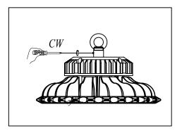
4). Make a circle of the lamp body with lifting rope , hang on the hook on the other side, and then ten sioning the lifting rope.
