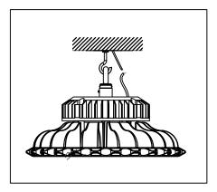
5).Connect those 3 wires(L: Black N: White G:Green) with correct cable, and turn on the power.
