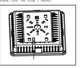
$\pmb{2}. Fix$  the bracket on J-box ,and put the wire through the central hole for wiring
