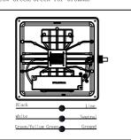
$2.\mathrm{Cut}$  off the wires through from  $3/4\mathrm{''}\mathrm{hole}$  and plug the hole with provided plug.Drill 4 holes on edge of fixture and fix it on the ceiling with using appropriate screws.
