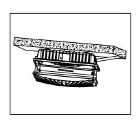
3.Remove 1/2" plug from direction you intend to feed conduit
