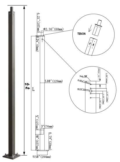
The Lapa Industries Straight Square Steel Light Poles are built from high strength steel tube and are available side drilled for arm mounted area lighting luminaires or with tenon mounts for flood and post top luminaires. Typical area lighting applications include retail centers, industrial parks, schools and universities, public transit and airports, office buildings and medical facilities. Mounting heights of 10 to 30 feet can be used based on selected luminaire application.
