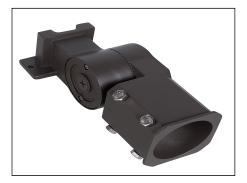
Slipfitter Mount An optional cast aluminum mast arm adapter secures fixture head to nominal 2"(2-3/8"O.D. pipe size) horizontal steel tenon arm.
