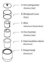
Put the wick(C) into the fire chamber(D). If solid fuel tablets are used, put them into the chamber directly without the wick, and skip step 4.
