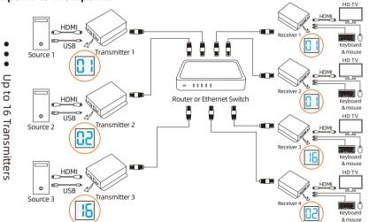
Support up to 16 Transmitters (communication ID: 1~16) in one local area network. Set the Receivers' communication ID to the same as the Transmitter which the Receiver wants to connect to.
