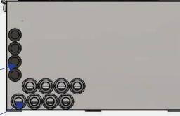
PG25 outdoor cable entry provision for IP55 ingress protection (8 no's)
