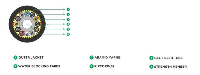
\* Typical Construction Diagram - Not to Scale
