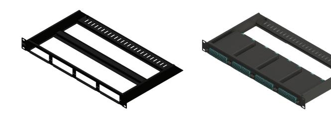
STL 1RU panel is a custom designed panel for MPO Cassettes. Made of CRCA steel sheet with black power coating, is very sturdy and provides long service life. Flat 1RU panel with 19 inch width is best suited for mounting inside the equipment racks. The rear cable support bar with slots for Velcro tie is the ideal solution to support and secure the connecting cable loop without any entangle with other adjacent cables.
