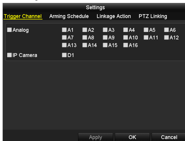
Figure 5. 20 Set Trigger Camera of VCA Alarm
