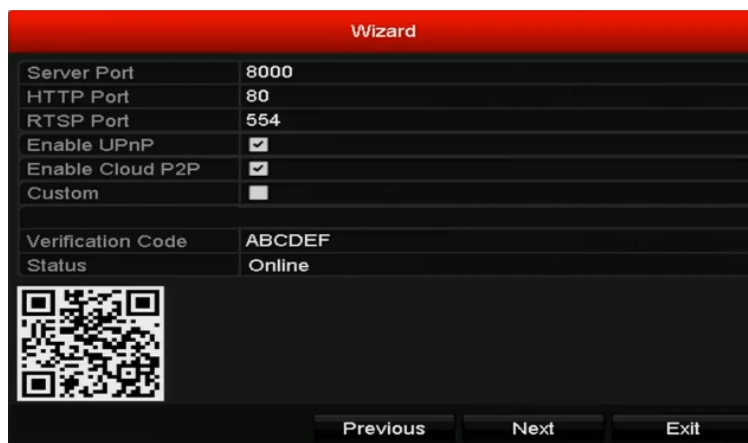
Figure 2. 8 Advanced Network Configuration
