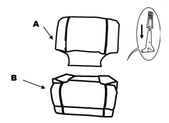
Step 2. Attach the arms to the both upper side of Step 3. Completed the seat, insert the arms and push to the end, make sure the brackets are secured in position.
