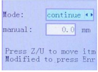
When Mode is selected, push or to choose between the two modes Continue and Manual. Push FN to move the cursor. When the cursor is on Manual, push or and A or V to change the
