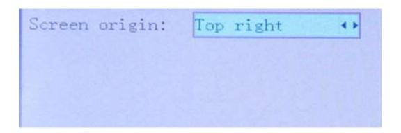
This interface sets the relative position of the origin. Different origin positions can generate different reflections of the graph over the X/Y axis. The operation method is the same as those described above.
