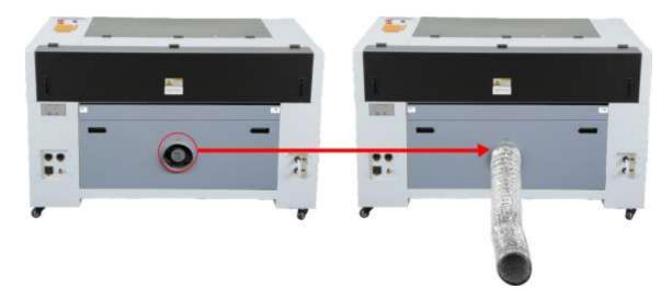
The other end should be connected to a dedicated purifier or (if the fumes are not hazardous and meet local and national air safety standards) placed out a window. NEVER operate the laser ifthe vent is not purifying or removing the fumes produced by the target material. Research materials before use and never operate the laser on any (such as PVC, teflon, and other halogen-containing substances) that can produce corrosive, hazardous, or even deadly fumes.
