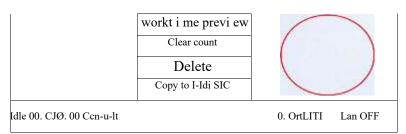
The system will automatically read the memory files. The file name and the work times will be listed and the selected file will be previewed in the upper right corner. Different memory files can be selected by using A or V . Press Enter to preview the selected file on the main interface. Press Esc to close the preview.
