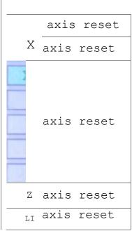
Push A or V to select an item. Press Enter to start the resetting of the selected axis, and the message "Resetting Is Underway" will show on the screen. Upon completion, the message will automatically disappear and the system will return to the main interface.
