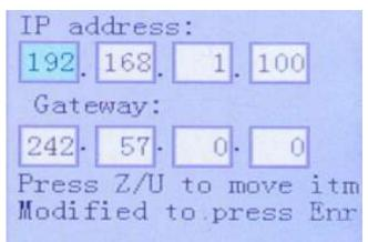
Press FN to select an item, and push or and A or V to change the parameters. Press Enter to save the changes or Esc to discard changes and return to the previous menu.
