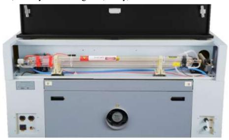
Step 4. Inside the main bay, remove the nylon cable ties from the X axis and the honeycomb table.
