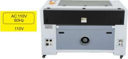
Fluxuation along the line should be less than 5%. If this is exceeded, the fuses will blow. They are located in the connection socket and are accessible from the exterior. Similarly, do not connect this device to standard extension cords or power strips. Connect it directly to a grounded outlet or use a surge protector rated over 2000J.
