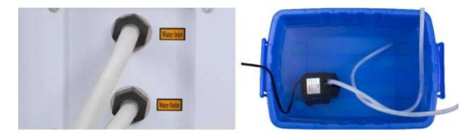
Connect the water pump to its power supply. For best results, use a power outlet on a separate fuse from the engraver itself. If no such outlet is available, the pump can also be plugged into a dedicated socket located on the side of the engraving cabinet. Once the pump is plugged in, water should begin to run through your machine and back into your tank. ALWAYS obtain visual confirmation that the water is flowing through the laser tube before starting your laser.
