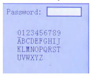
Push or and ▲ or ▼ to select a password and press Enter to save it. The current parameters of the machine will be stored as its defaults. They can then be retrieved by using the Restore Default Parameters command. It is recommended that you save your machine's actual factory default settings, so they can be easily restored when need be.
