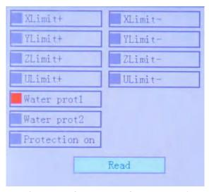
This interface contains input/output information of the system's hardware. Press Read Para to access hardware information. When the hardware signal is triggered, the small box to the left of the corresponding item will be displayed in green, otherwise it will be grey. Press Esc to return to the previous menu.
