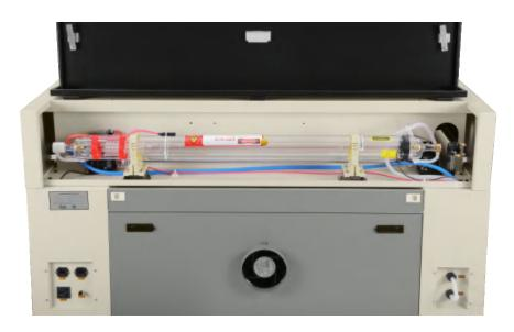
**Step 4.** Inside the main bay, remove the nylon cable ties from the X axis and the honeycomb table.
