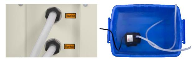
Connect the water pump to its power supply. For best results, use a power outlet on a separate fuse from the engraver itself. If no such outlet is available, the pump can also be plugged into a dedicated socket located on the side of the engraving cabinet. Once the pump is plugged in, water should begin to run through your machine and back into your tank. **ALWAYS** obtain visual confirmation that the water is flowing through the laser tube before starting your laser.
