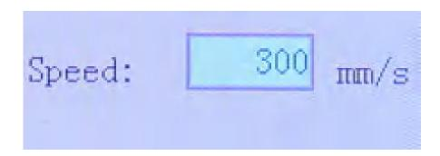
A cursor will appear when pushing or . Move the cursor to the numeral area and push ▲ or ▼ to change the value. Press Enter to save the change. Press Esc to invalidate the change and return to the main interface.
