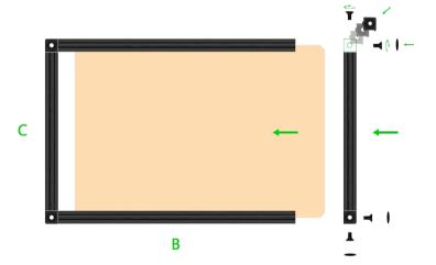
b. Insert the top panel along the groove of the aluminum profile frame, and finally assemble the unassembled side aluminum profile, aligning its groove with the acrylic panel, so that the complete top part can be assembled.
