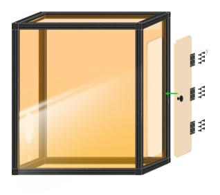
® Align the hinge with the hole of the door and fix it with screws, install the door.
