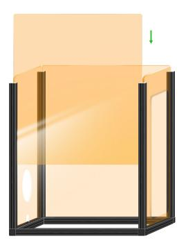
4 Insert the four side panels along the grooves of the aluminum profile
