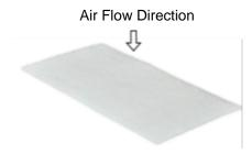
Use method: Place the Pre-filter on top of Middle Filter. The front side (rough side) is facing upwards (air inlet direction). When the accumulated dust on the Prefilter is over 70% and cannot be cleaned any more, please replace the Pre-filter with a new one.
