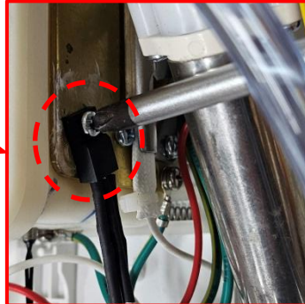
④ Use screw 1EA to connect the triac of the replaced MAIN PCB with the TANK.
