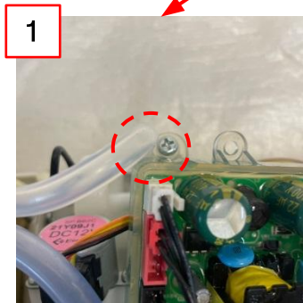
① Check whether the nozzle hose is caught on the MAIN PCB.
