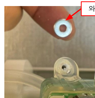
② Separate the screws of the MAIN PCB, insert a washer between them, and reassemble.
