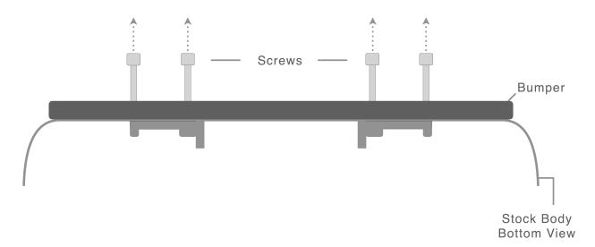
Insert your new rear lights between the body and mount. Align the screw holes and reinstall the factory screws.
