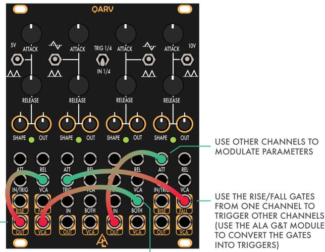
CREATES AN EXPONENTIAL -SIGNAL OUTPUT FROM THE VCA (OUT KNOB CONTROLS VOLUME)
