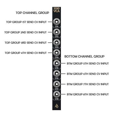
THE SEND KNOB ON EACH CHANNEL ACTS AS A "MAX VOLUME" KNOB WHILE A CABLE IS INSERTED INTO IT'S SEND VCA CHANNEL. POSITIVE VOLTAGE WILL OPEN UP THE VCA AND WILL HIT THE "MAX VOLUME" LEVEL AT 5V.
