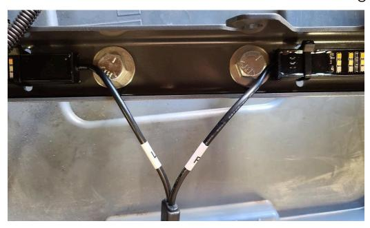
Press down on light with your fingers to set the adhesive. Install (4) zip ties at ends for security.
