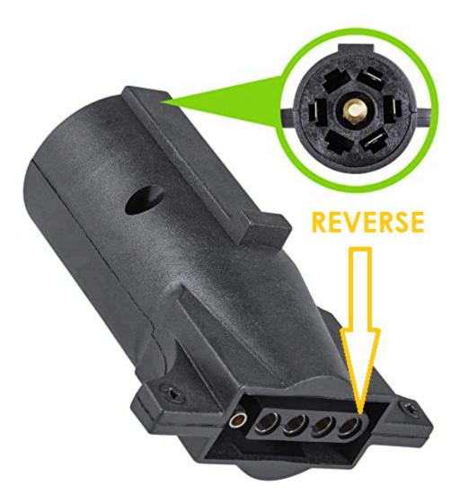
Plug in the single loose wire to the plug as shown for reverse light operation.
