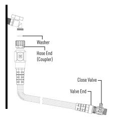
Water pressure must be 60 PSI to get optimal performance and expansion.
