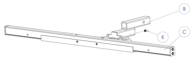
2. Place a 3/8" WASHER on bolt and slide through beam (Part C) and hitch adapter (Part B)
