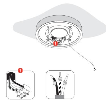
Pay attention to the labels that identify exactly the wires: Line, Ground, Neutral
