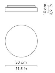
Wall-ceiling lamps with diffuser in mouth-blown, satin-finish opal triplex glass, and white painted metal frame. Twist-lock system for the glass component. The product is suitable for indoor use only.
