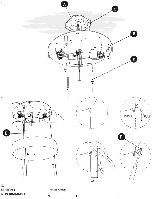
1. The canopy is made up of a back plate with the electrical connections on it and a front cover.
