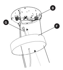
**4.** Now take the 3 cables coming from the lamp (E), and feed them through the canopy cover (F) and make the connections to the driver in the canopy (B) as indicated at point 5.
