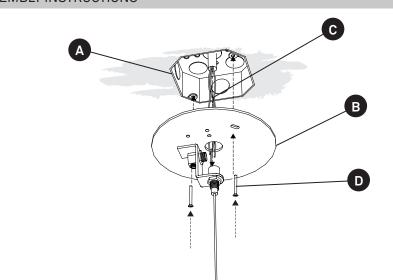
**1.** The canopy is made up of a back plate with the electrical connections on it and a semi spherical cover.
