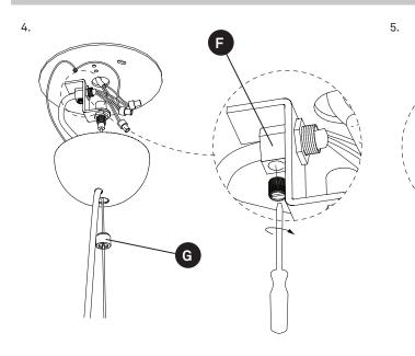
4. Tighten the screw on the electrical cable trap (F).
