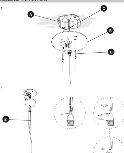
**1.** The canopy is made up of a back plate with the electrical connections on it and a semi spherical cover.
